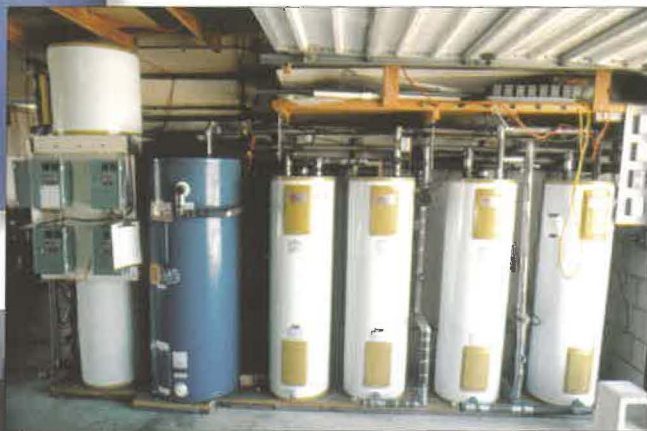
Tom Tiedemann's Solar Hot Water tests for storage tank configurations
