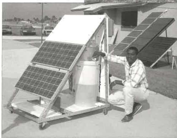
M. Keita, with small-scale PV powered reverse osmosis desalination unit (October 1990)
