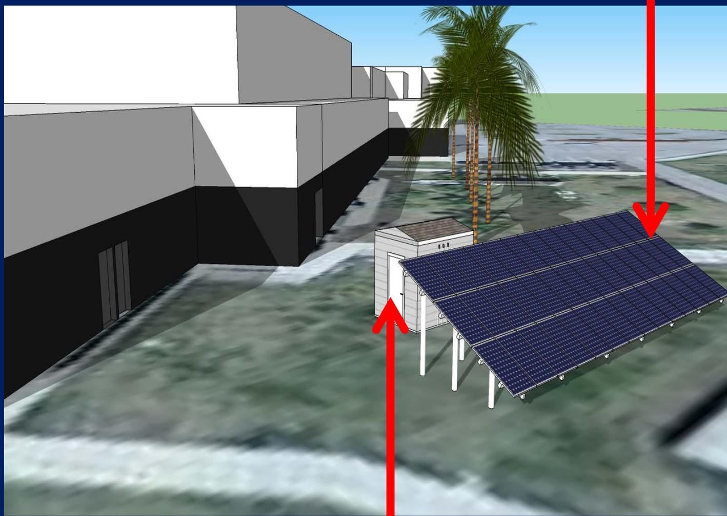
The SOLAR EQUIPMENT ENCLOSURE houses the inverters, batteries, and charge controllers.
