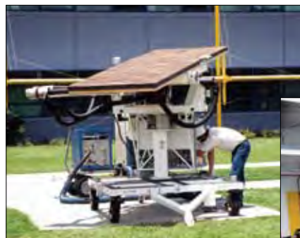
Solar collector being tested on mobile test platform (March 2000)
