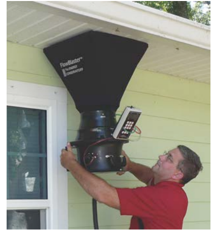
FSEC specializes in all aspects of building science, including indoor air quality. Mechanical ventilation testing is shown here.
