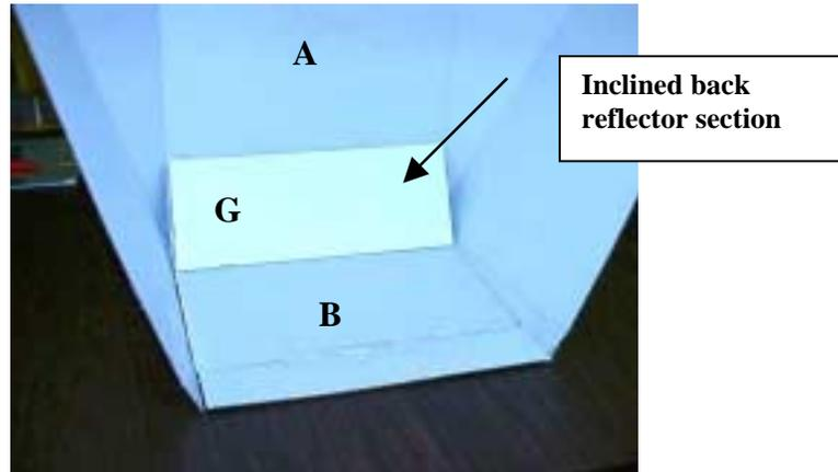
Note that the “inclined back section” will be folded against the back panel when the unit is closed for storage and transport.
