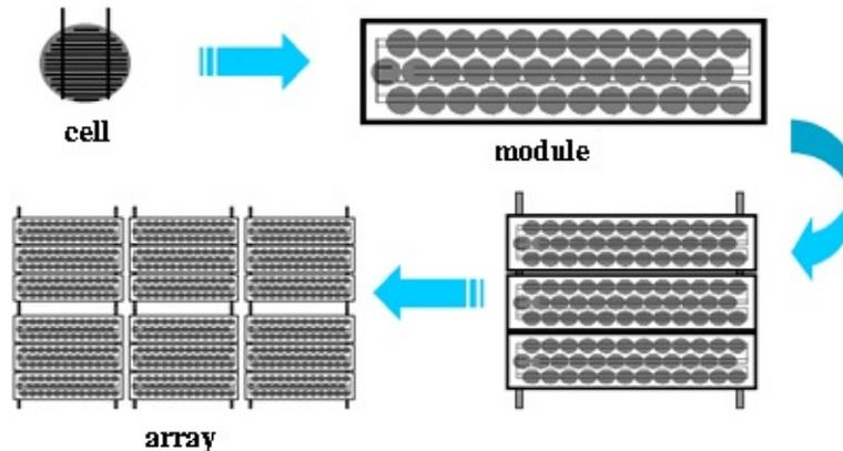
The **photovoltaic array** which is made up of several photovoltaic modules, converts sunlight directly into electric current. Like batteries, the current they produce is direct current (DC).
