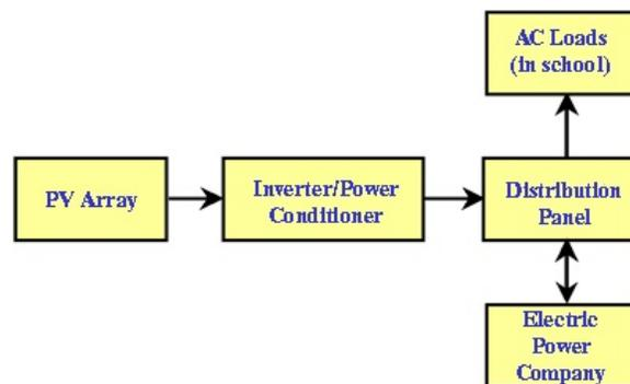
The **inverter** changes the DC electricity produced by the modules into alternating current (AC) which is the type of electricity used in your school and home.
