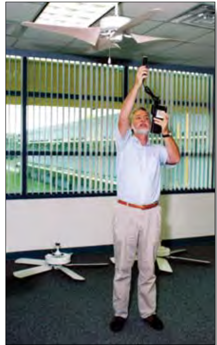
Danny Parker measures air speed from patented "Gossamer Wind" ceiling fan (October 1998)
