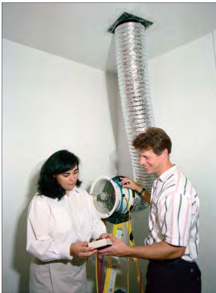
Janet McIlvaine and Rob Vieira conducting duct leakage test (October 1998)
