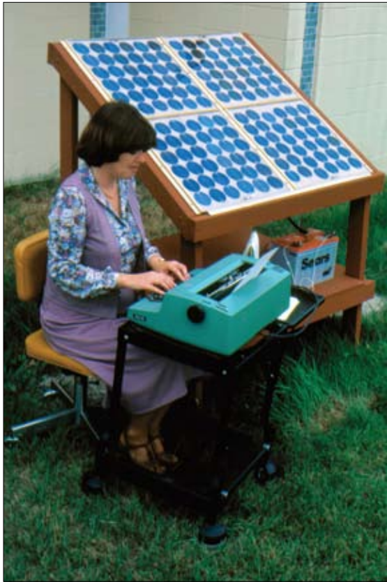
Carolyn Burby at FSEC's first 40-watt PV system, used to power typewriter (October 1978)
