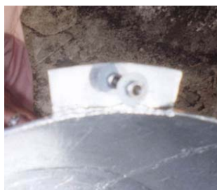
While focusing, shadow of upper washer adjusted towards west
