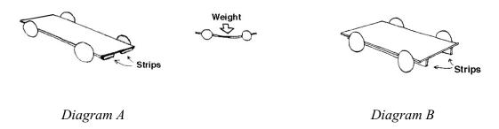
12. In the diagrams above, which method of bracing will result in the stiffer chassis — diagram A with the bracing flat in relation to the chassis, or diagram B with the bracing on edge in relation to the chassis? To find out, use a ruler to simulate the bracing and try and bend it downwards while holding it (at the ends) first flat like in diagram A, and then on edge like in diagram B. Which way was it the hardest to bend the ruler?
