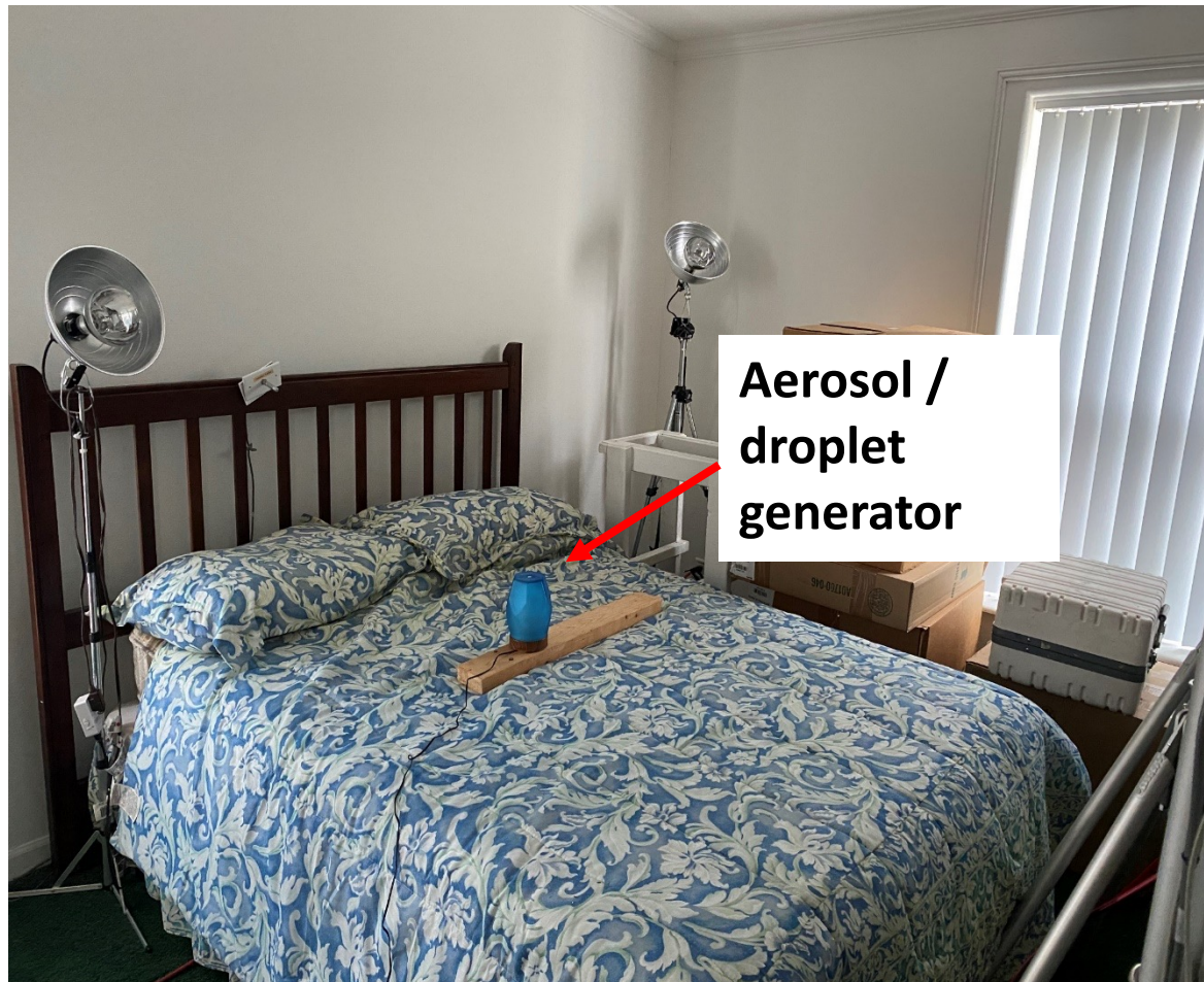
Fig. 3. Aerosol concentration measurements are taken in the isolation zone and in the main zone simultaneously.
