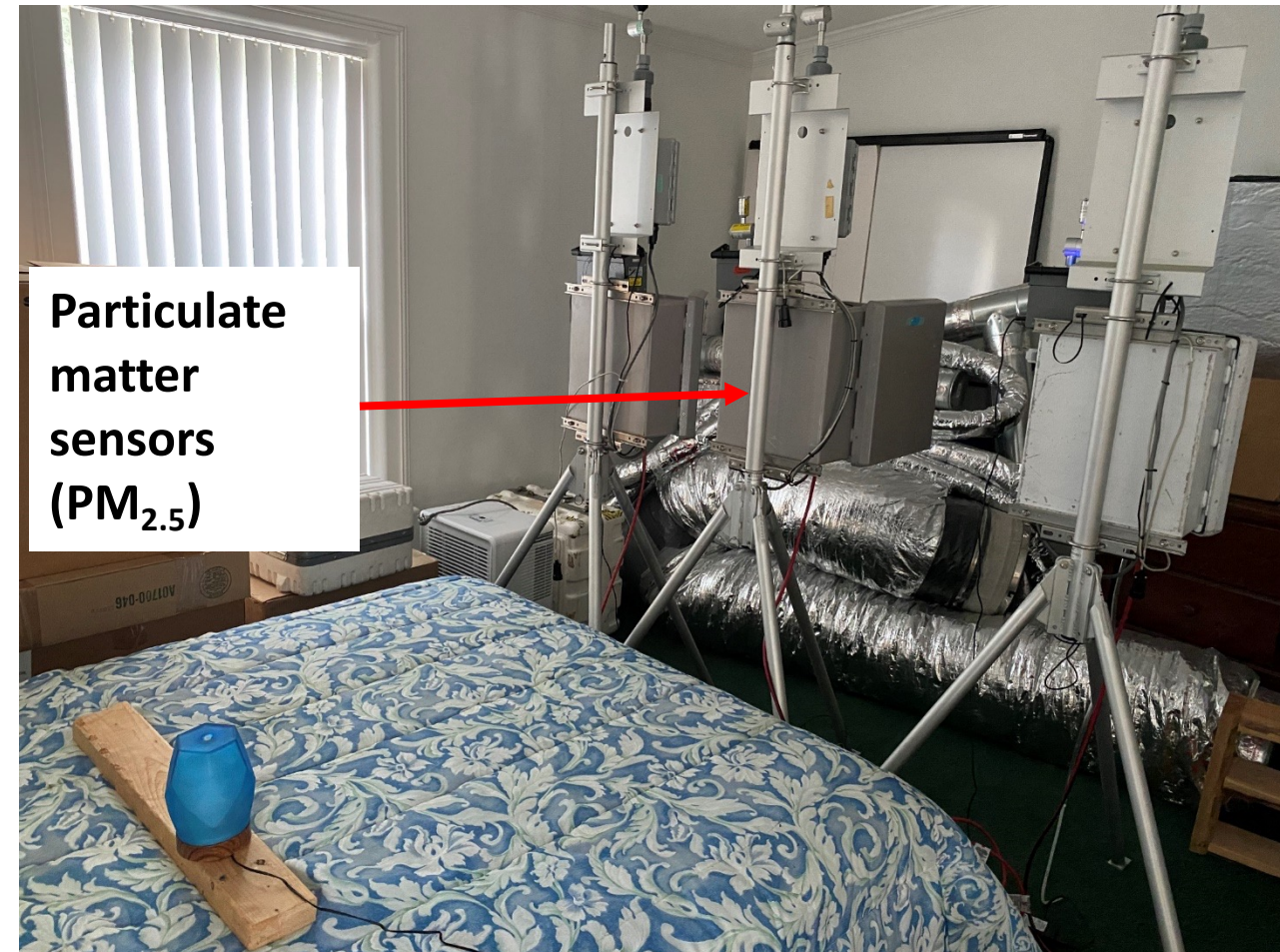
Fig. 3. Aerosol concentration measurements are taken in the isolation zone and in the main zone simultaneously.
