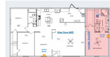
Figure 1. The FSEC Manufactured Housing Lab was used for experimentation with the master bedroom (pink) used for the isolation zone and the living room used as the safe zone, or main zone. Image courtesy of FSEC.
