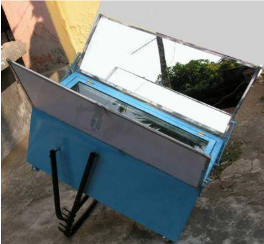
A box cooker built from a repurposed cabinet and mirrors
