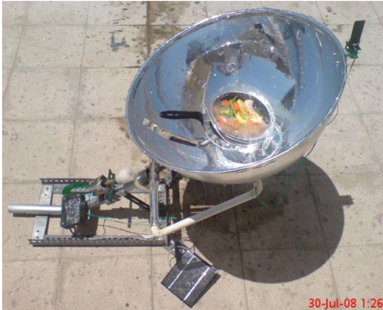
A deep parabolic with a photovoltaic powered tracking system
