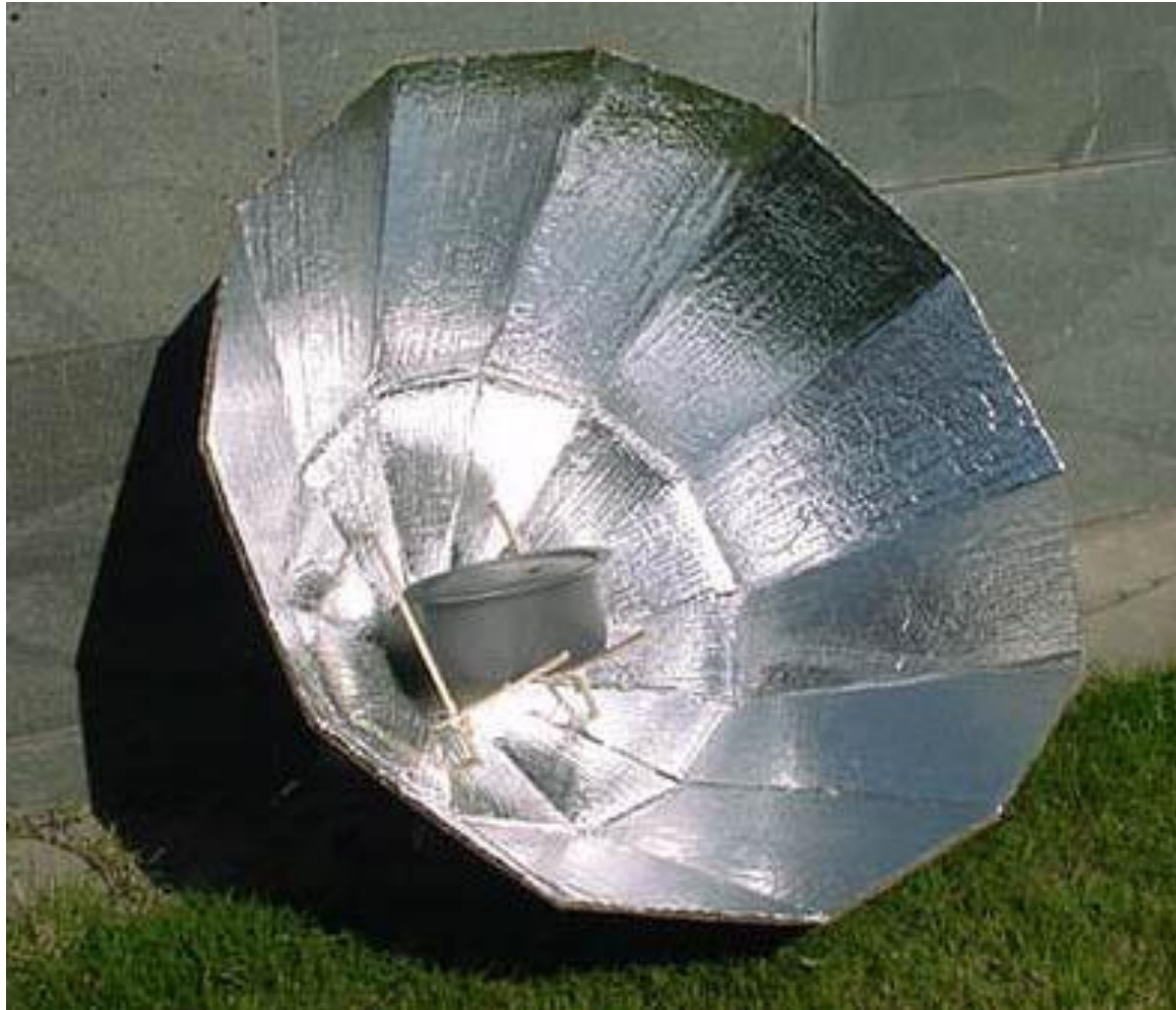
An inexpensive cooker made from cardboard, mylar, glue and some wooden dowels
