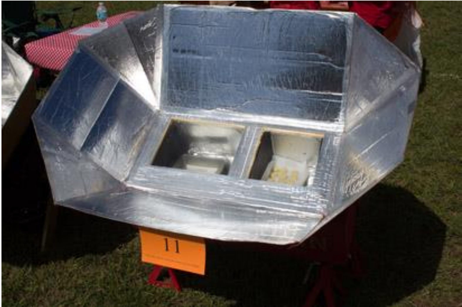
A student designed box cooker with 2 chambers
