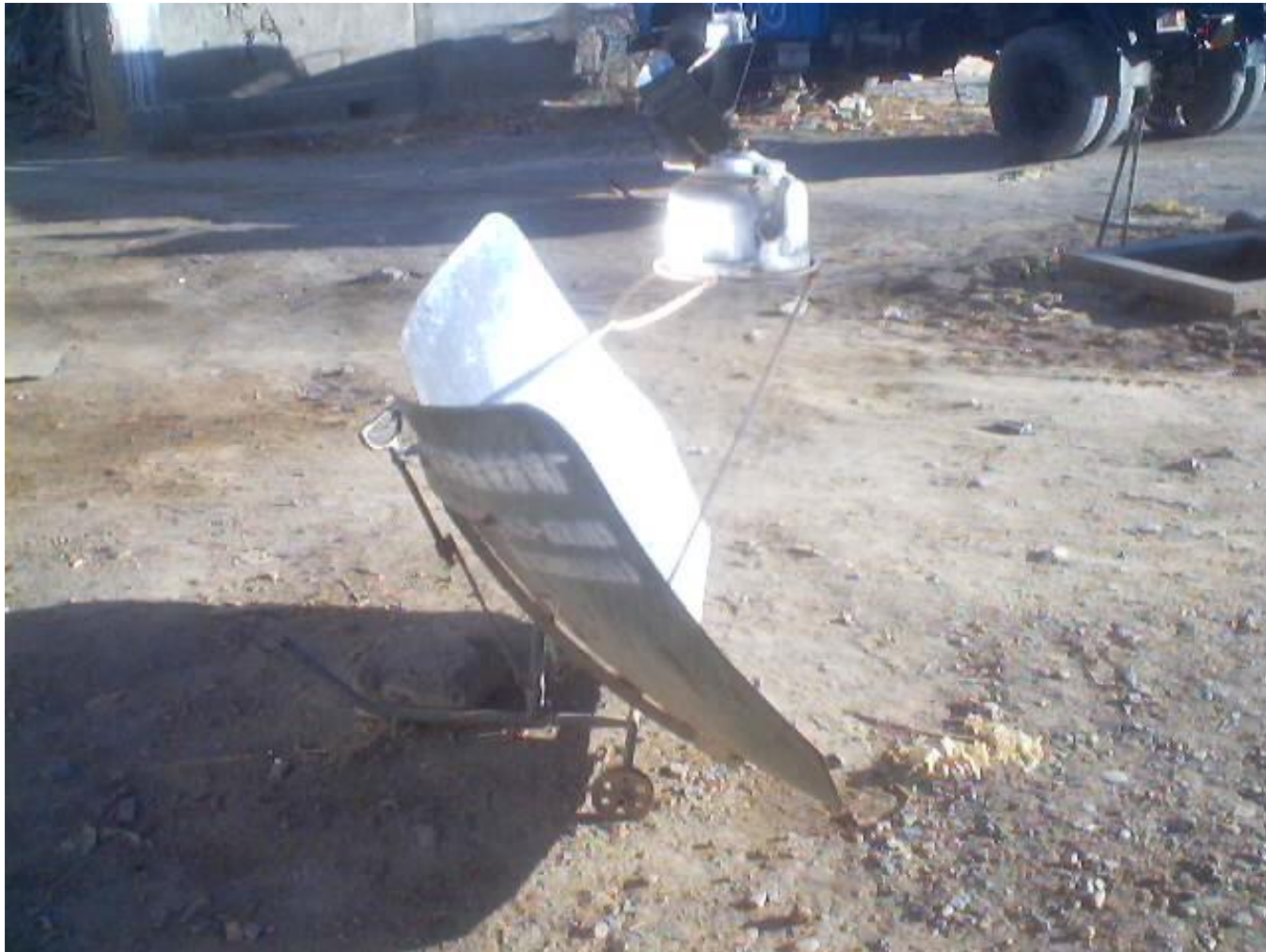
A commercial panel cooker that can be wheeled into place
